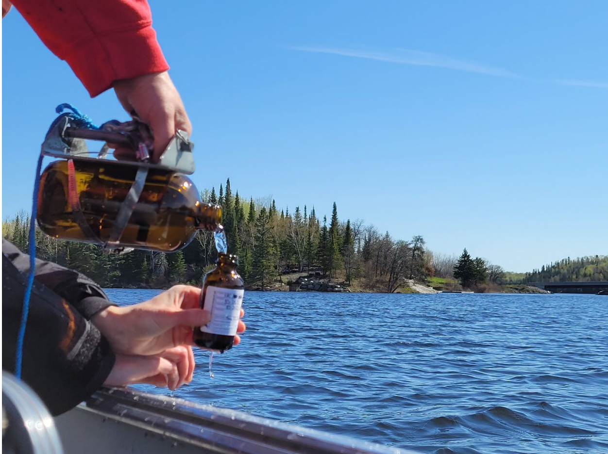
Figure 4 – Transferring water sample from euphotic zone composite into lab sample bottle
