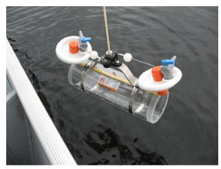
Figure 4 – Horizontal Beta Sampler prior to deployment
