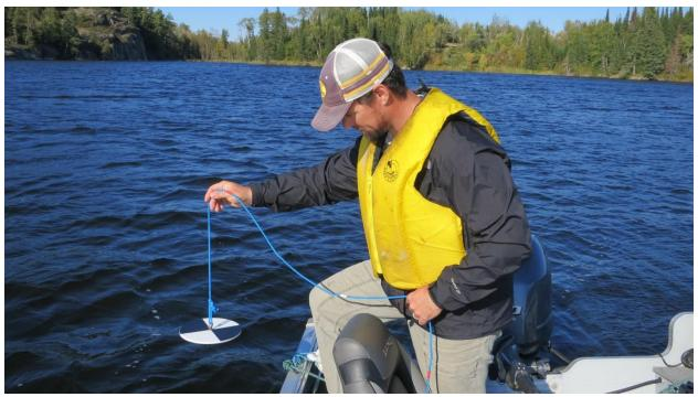
Figure 2 – Lowering of Secchi disk
